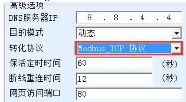
Figure 19 start Modbus TCP function
