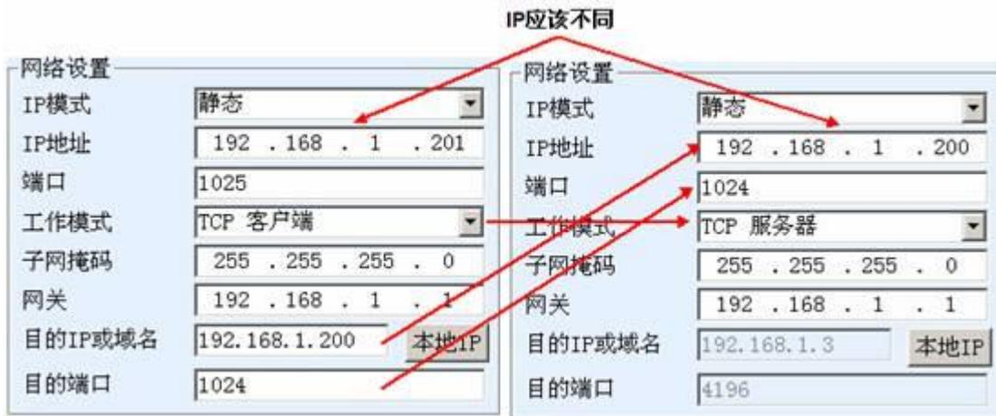
Figure 24 TCP Configure device couplet parameters
