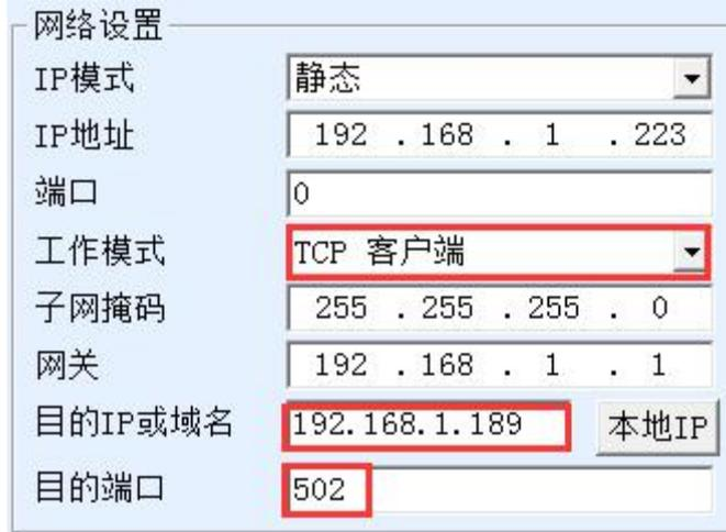
Figure 20 Modbus TCP being client side
