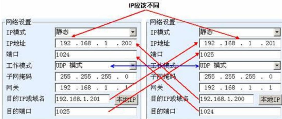
Figure 26 UDP Configure device couplet parameters
