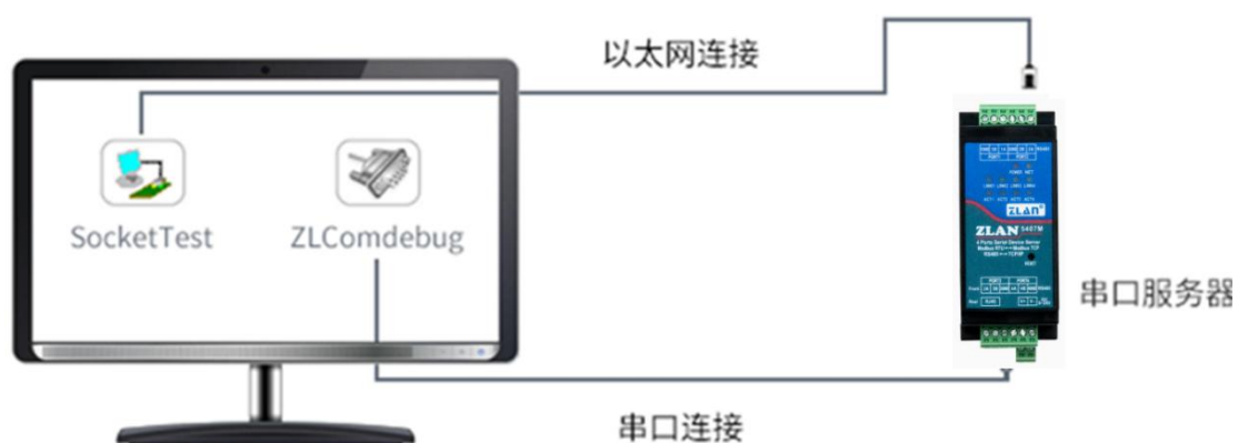
Figure 9 TCP communication diagram
